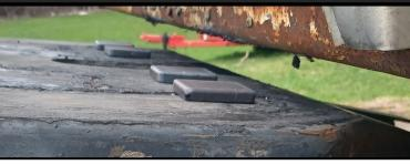
Trailer edge should contact upper end of 5<sup>th</sup> wheel Pads should be well under trailer
