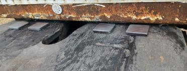
Trailer clearance should be sufficient to allow the pads to pass under the trailer without contacting
