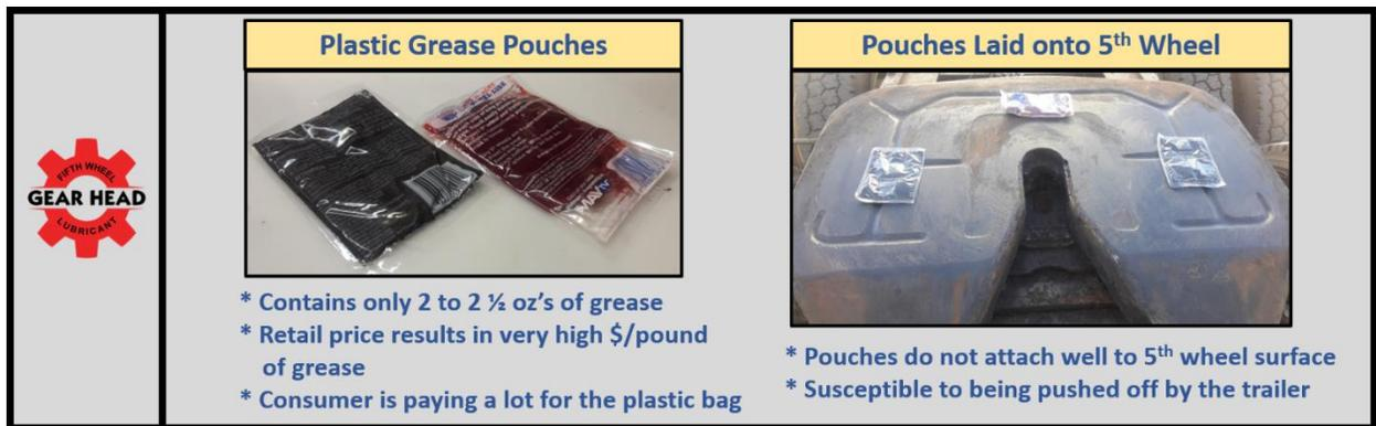
Unfortunately, at some point the baggie will either be pushed out of the joint; or will fall off the trailer surface onto the ground when the trailer is sitting and not connected to a truck. In either case, the baggie becomes a serious source of litter on the roadways and in parking lots. One wonders why this type of product should even be available in the marketplace.
